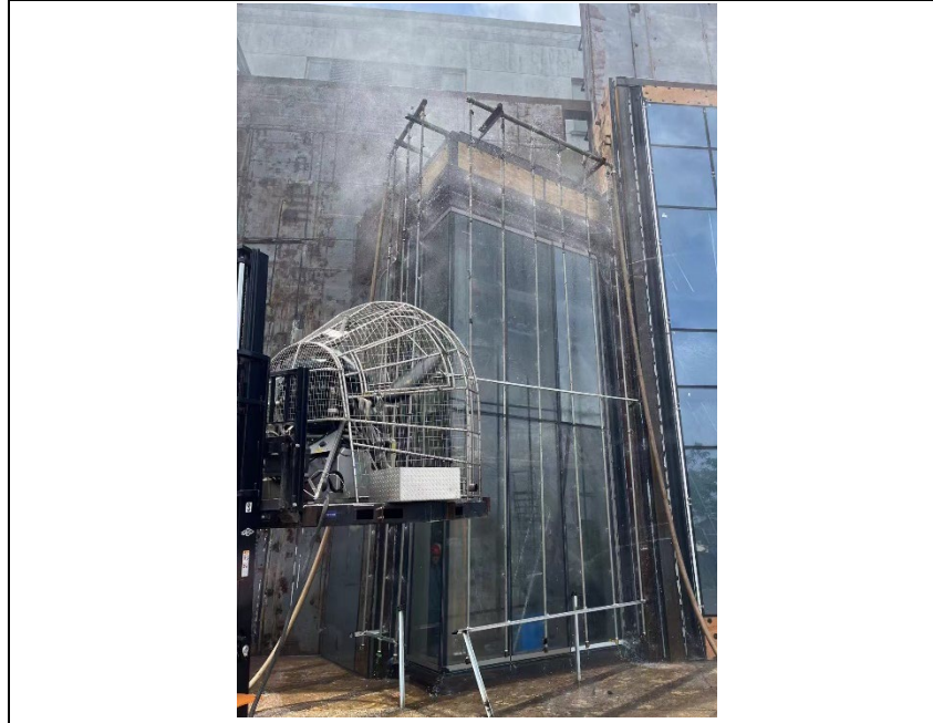
Photo No. 3 Dynamic water penetration test-Specimen #12
